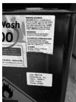
Fig. 6 - Solvent missing safety information.
